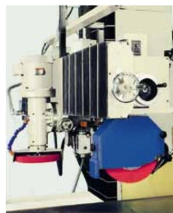
**Vertical Spindle Grinding Equipment**
